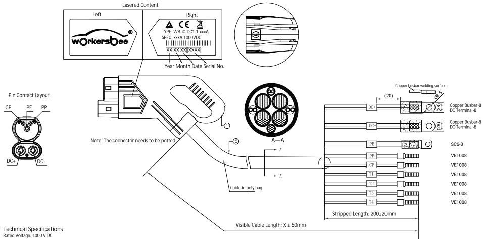
Rated Current: 250A, 300A, 350A, 375A Ambient Temperature: -30°C to +50°C Cooling method: Natural cooling
